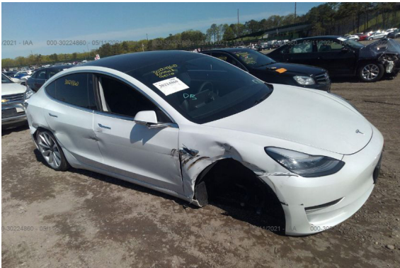
This image from the website stat.vin, which tracks car auctions, shows a 2020 Tesla Model 3 that was damaged in an April 2021 accident. The vehicle's front wheel fell off while driving at 60 mph, according to a Tesla technician's summary of the incident.
